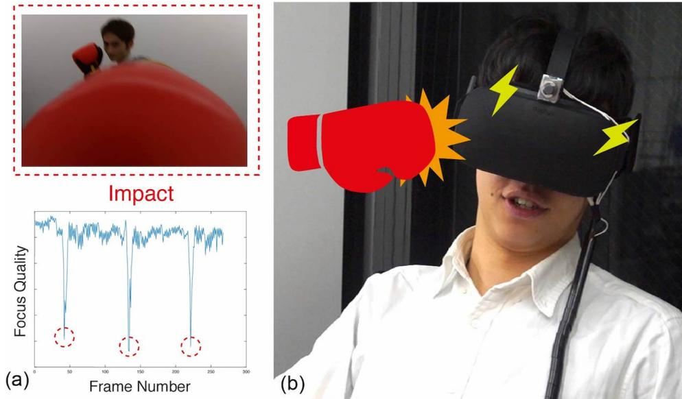
Figure 6.2: An experience being punched in the face. (a) A significant blur is recognizable at the timing of impact. In the video, 3 punches were performed in 9 seconds, recorded at 30 fps. (b) When the punch lands on the user’s face, In-Pulse stimulates the user for feedback.
