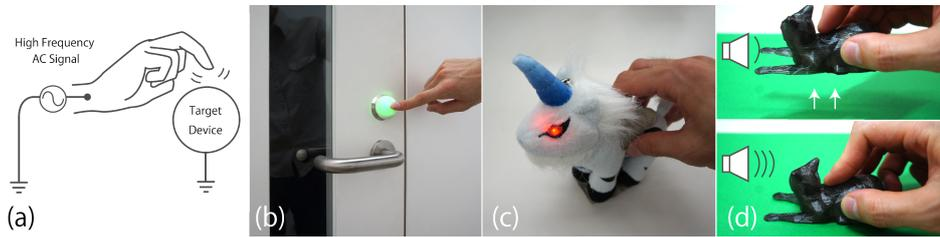
Figure 7.1: Intentiō and its applications: (a) Intentiō enables users to distribute power to electronic devices from power passing through their body. (b) Electronic and IoT devices are activated and powered by power distributed from the user. (c) Electronic stuffed toy activated by the user. The LED eyes emit light when the user touches the toy. (d) The user can adjust the amount of power distributed to the target device. Here, the volume of an electric music box is being adjusted.
