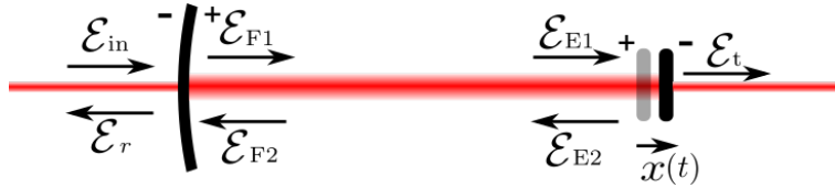
Figure A.6: Schematic view showing a Fabry-Perot cavity. \mathcal{E}_{\text{in}} , \mathcal{E}_r , and \mathcal{E}_t are the electric fields of the incident, the reflected and the transmitted light, respectively. \mathcal{E}_{F1} , \mathcal{E}_{F2} , \mathcal{E}_{E1} , and \mathcal{E}_{E2} are electric fields inside of the cavity.
