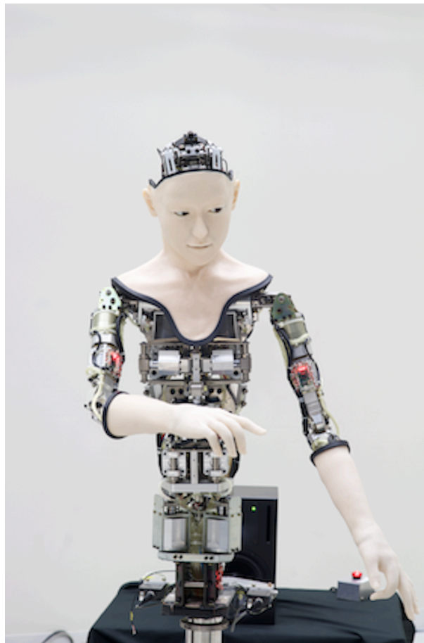
Figure 6.14: The appearance of the humanoid robot: Alter. The body was fixed to a pedestal. The total height is approximately 155 cm. (Photo by Kenshu Shintsubo.)
