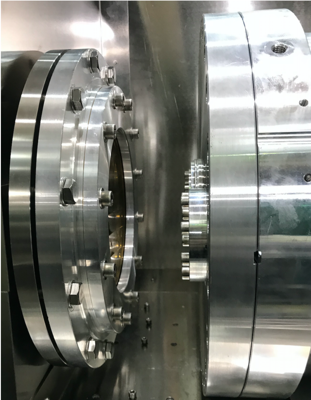
Figure 3.5: A pipe duct for beam extension (left). The duct end is covered by a sheet of 75 \mu\text{m} polyimide film. The distance between the duct end and the foil on the gas chamber (right) is 10 cm.
