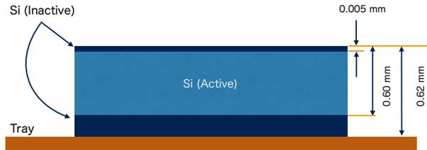
Figure 6.4: Inactive layers in Si detectors.
