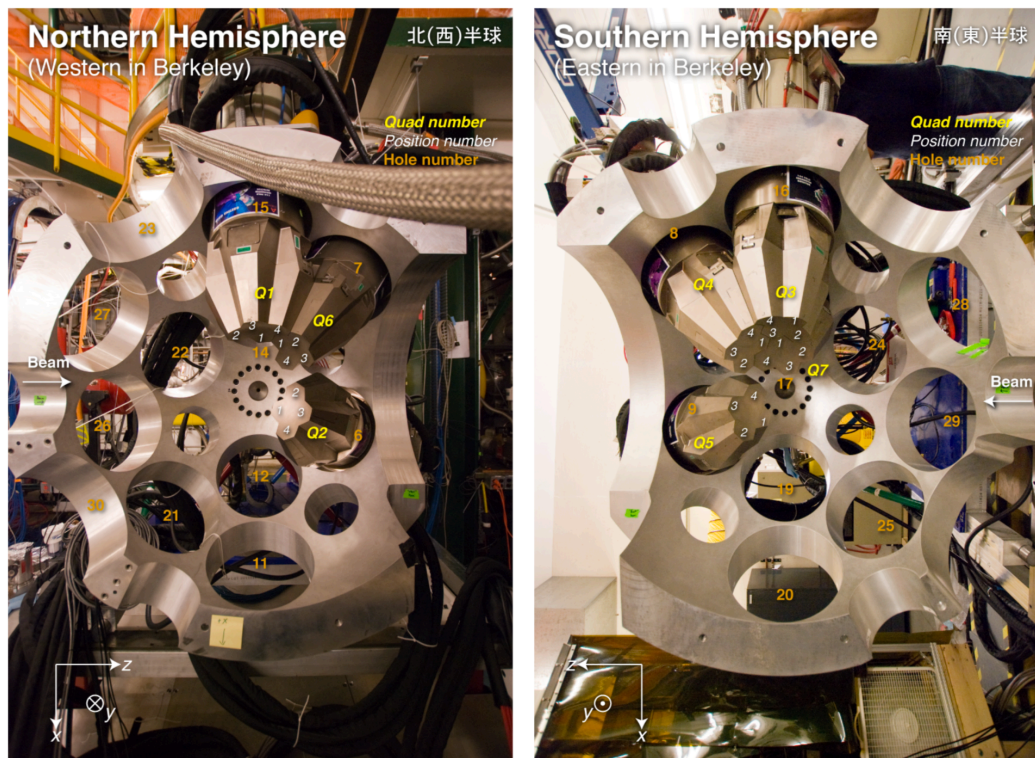
Figure 3.6: Picture of the GREY-TINA mount. In this picture, orange numbers represent the hole number, yellow numbers are the quad number, and the white numbers are the crystal number of each quad. Note that this picture was taken in the previous GREY-TINA campaign (2012). In the present experiment, 8th quad was additionally mounted in the hole 14. Taken from [67], picture courtesy of S. Noji.
