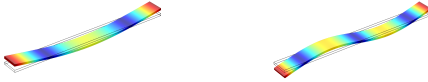
Figure 4.4: Shapes of the bending modes of the bar mirror whose length is 15 mm. The left (right) shows the first (second) bending mode. These are results from the finite element analysis by COMSOL. The red area means that the amplitude of the oscillation is large, and the blue area shows the node.
