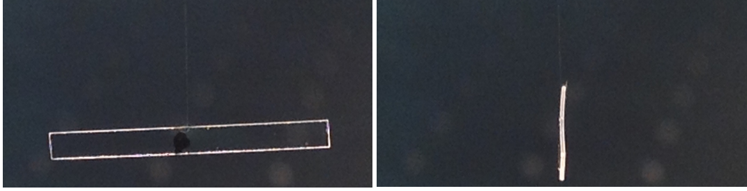
Figure 4.5: A photograph of the bar mirror from the front and side views. Our test mass seems to be warped at the mirror coating. The curvature is measured to be around 200 mm.
