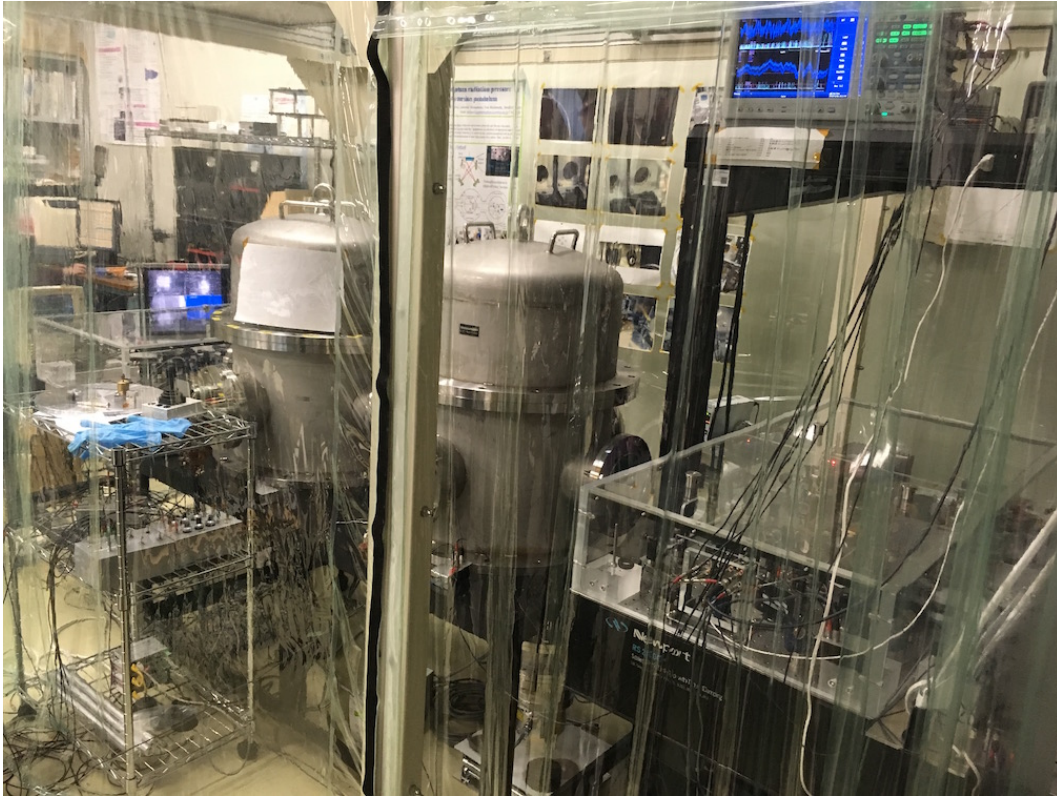
Figure 4.33: A photograph of the entire apparatus of our setup. The apparatus consists of the input optical table, the first vacuum chamber including the intensity and frequency stabilization system, the second chamber containing the main cavities, and the associated optics from the front to the back. The time series data are recorded in a logger at the right top. We see outputs of the CCD cameras with a monitor for the cavities resonance.
