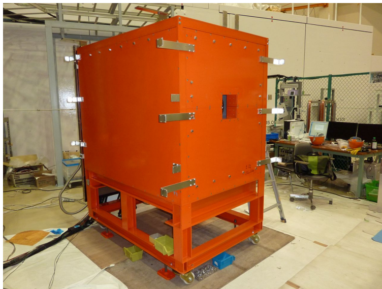
Figure 2.12: Picture of lead shield surrounding the TPC [21]. The thickness is 10 cm for the front side and 5 cm for the other five sides, respectively.
