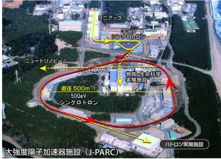
Figure 2.1: Bird's eye view of J-PARC [17]. Proton beams are accelerated by three types of accelerators: 400 MeV linear accelerator, 3 GeV rapid cycle synchrotron, 50 GeV main ring.
