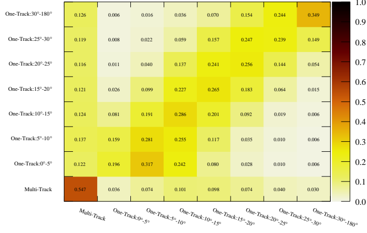
Figure 7.1: Product of the smearing matrix on scintillators of WAGASCI and U-Matrix on Proton Module, \sum_i \mathbb{P}(X_j^{\text{reco}}|C_i^{\text{true}})_{\text{WM}}^{\text{CH}} \times U_{ij'}^{\text{PM}} .
