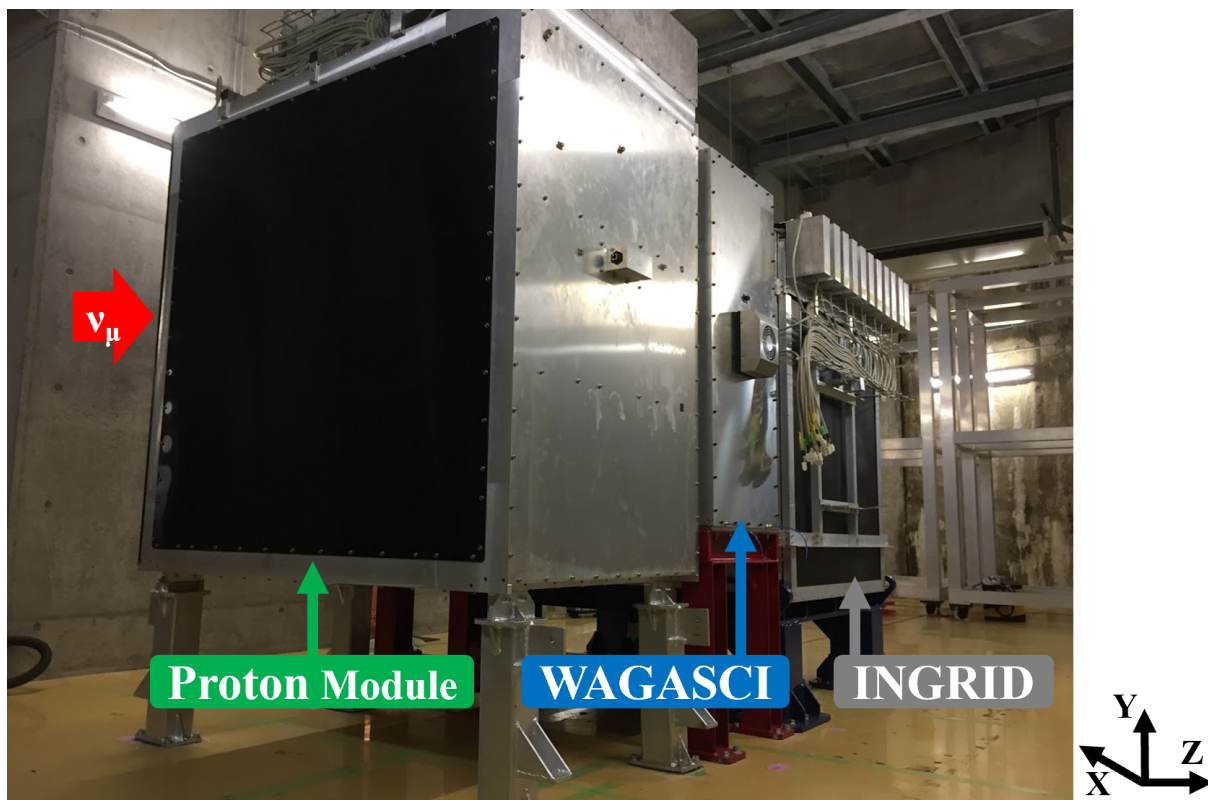
Figure 1: Installed detectors at the B2 floor in the J-PARC neutrino monitor building. The coordinate system used in this note is shown: The beam axis corresponds to Z axis.
