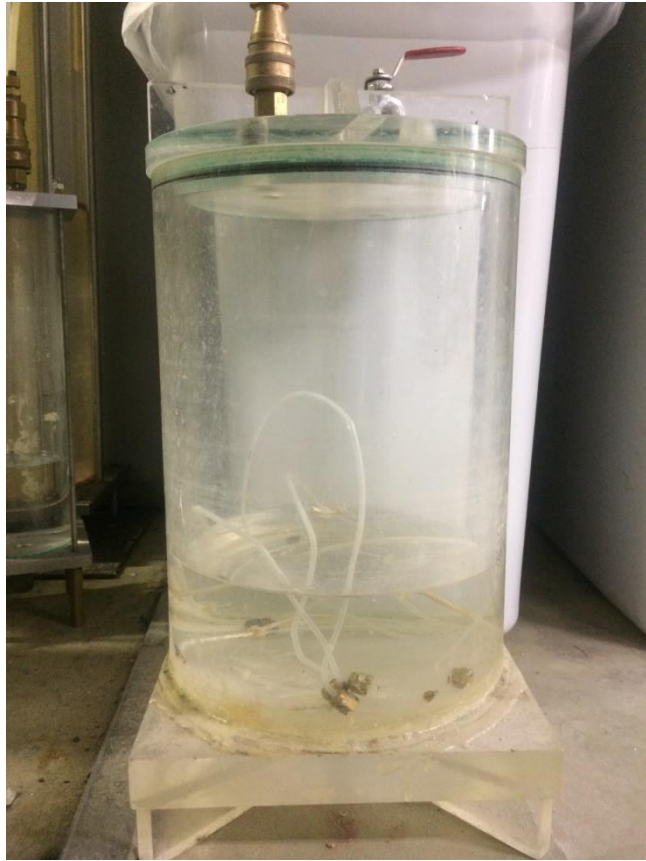
Fig. 4-56. Local pin-type sensors submerged in a tank with pressure of -100 kPa
