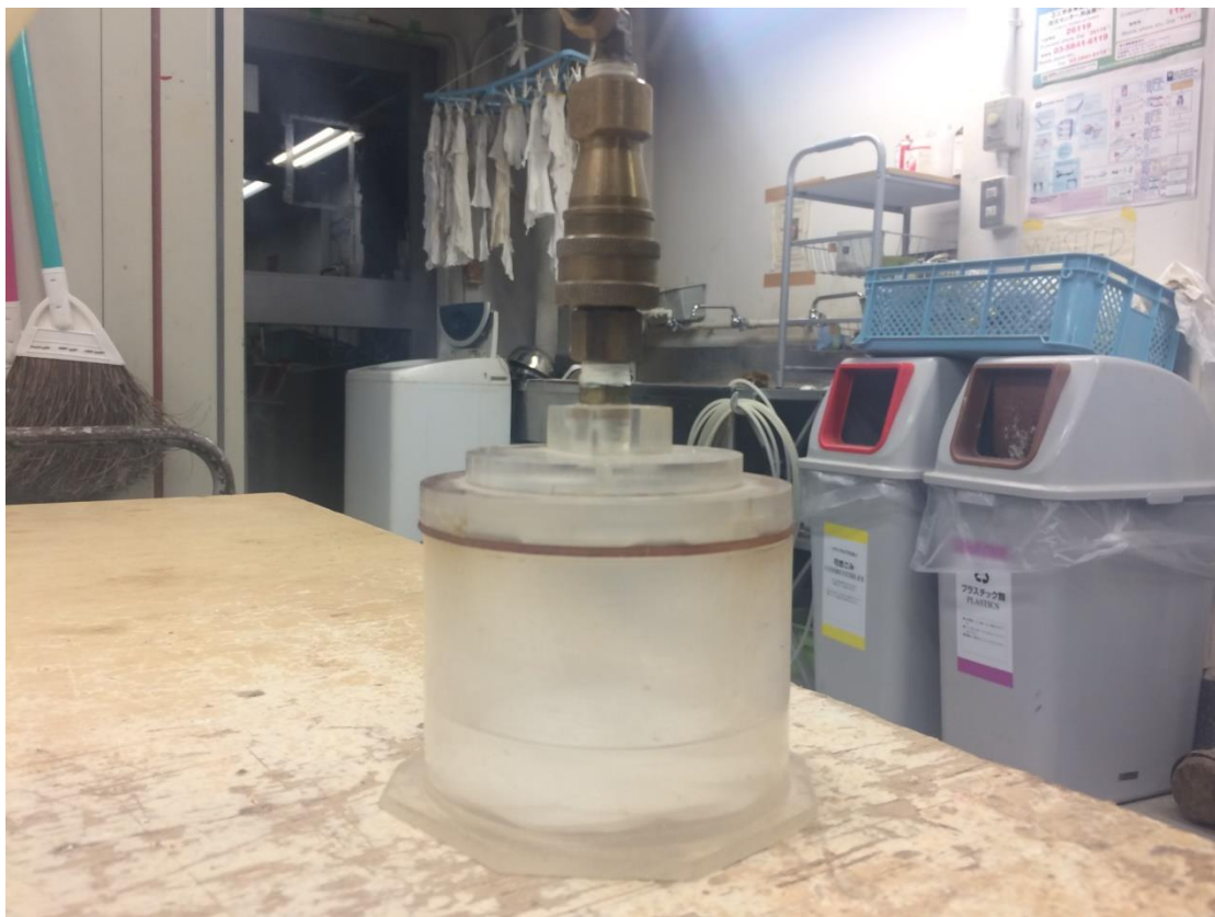
Fig. 4-57. Membrane filters being saturated in a container with pressure of -100 kPa
