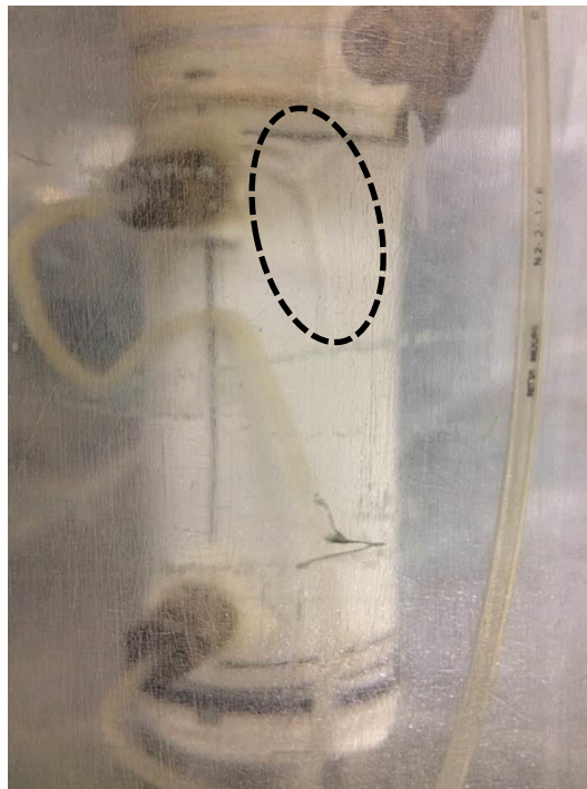
Fig. 4-16. Snapshot of specimen at 5 kPa showing membrane wrinkle (Toyoura sand test 5 – saturated)
