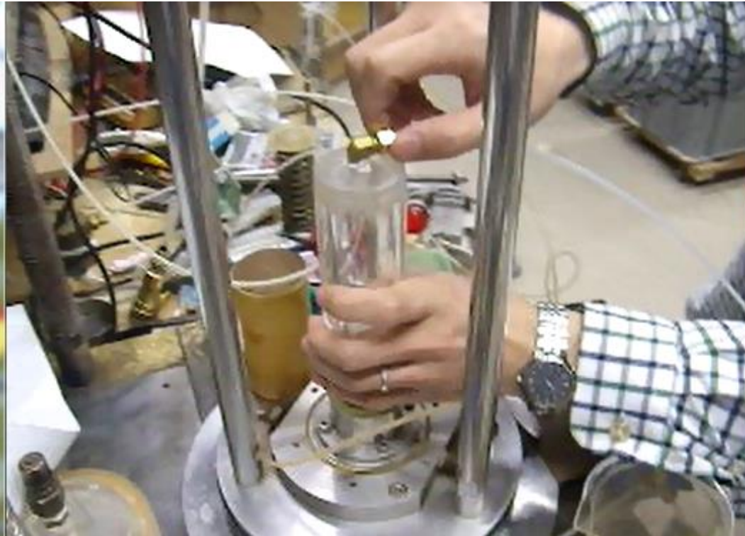
Fig. 3-29. Water-tight acrylic pipe used to saturate the bottom pedestal
