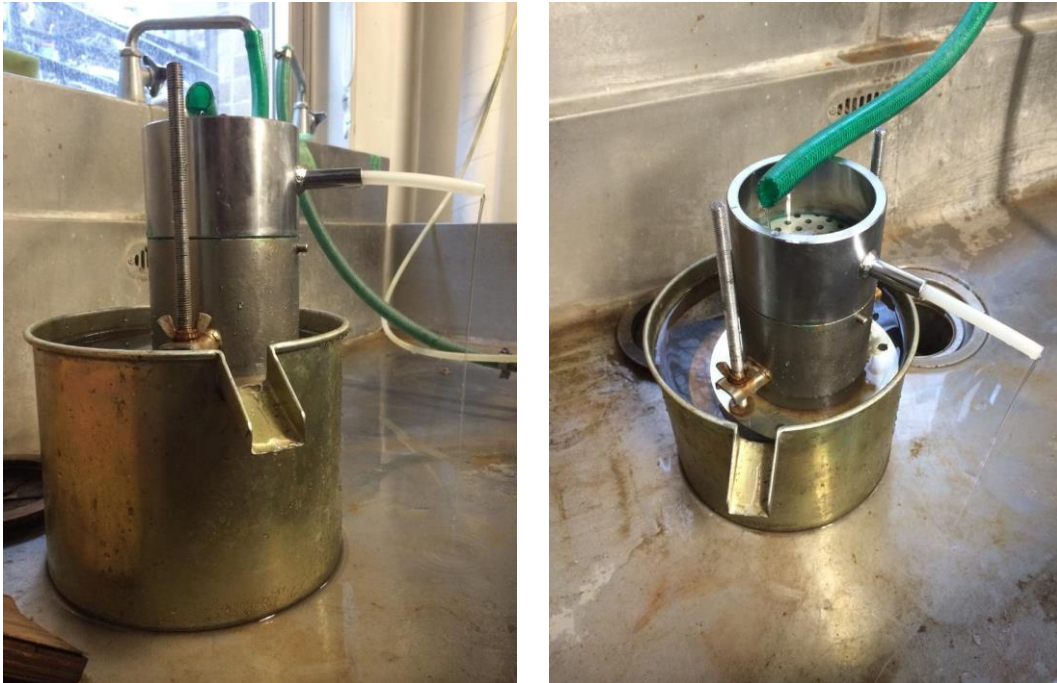
Fig. 4-3. (Left) Front view of Permeameter test set-up at 12 cm head; (Right): Top view
