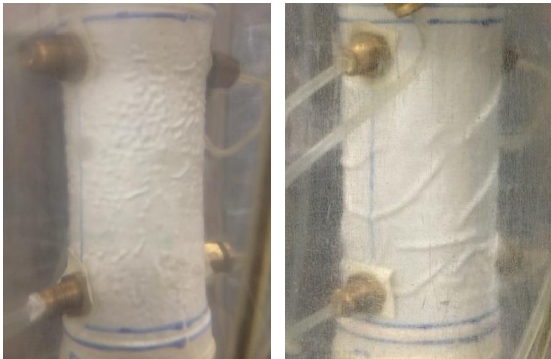
Fig. 4-14. Snapshots of specimen at 20 kPa (left figure) and 10 kPa (right figure) showing membrane wrinkle (Inagi sand test 3 – saturated)
