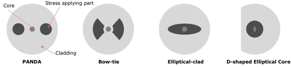
Fig. 3.3. Different types of polarization maintaining fibers.
