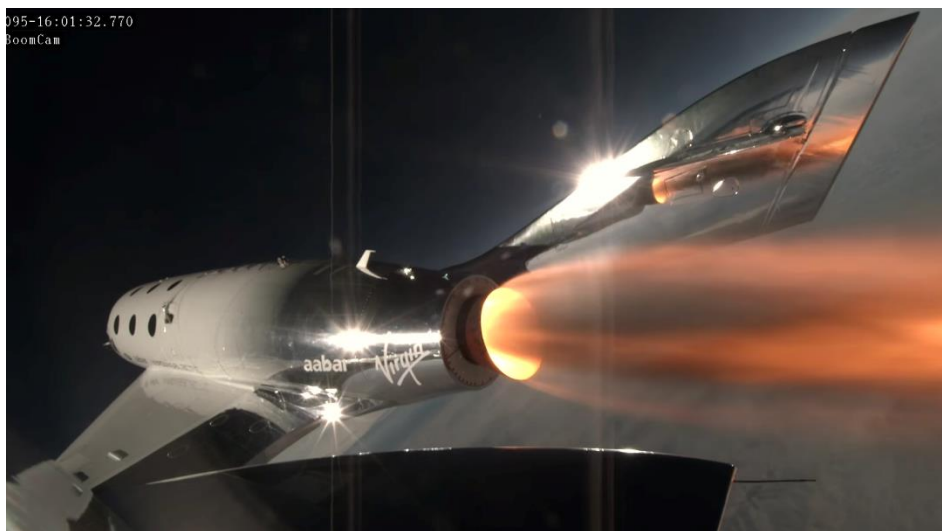
Fig. 1.3 Hybrid rocket in operation during the flight test of the VSS Unity [1-4]
