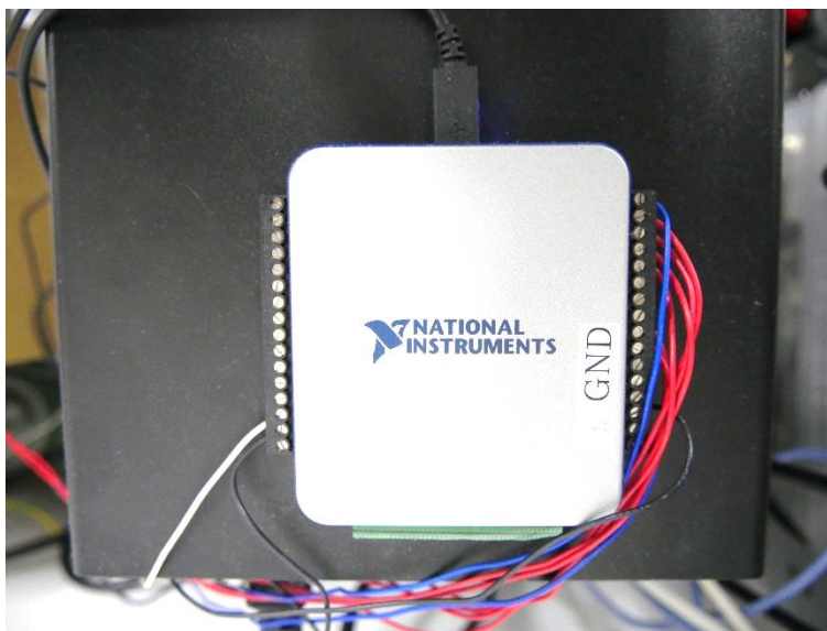
Figure 2-25 Photograph of the DAQ I/O device for LabVIEW (NI, model: USB-6001) .
