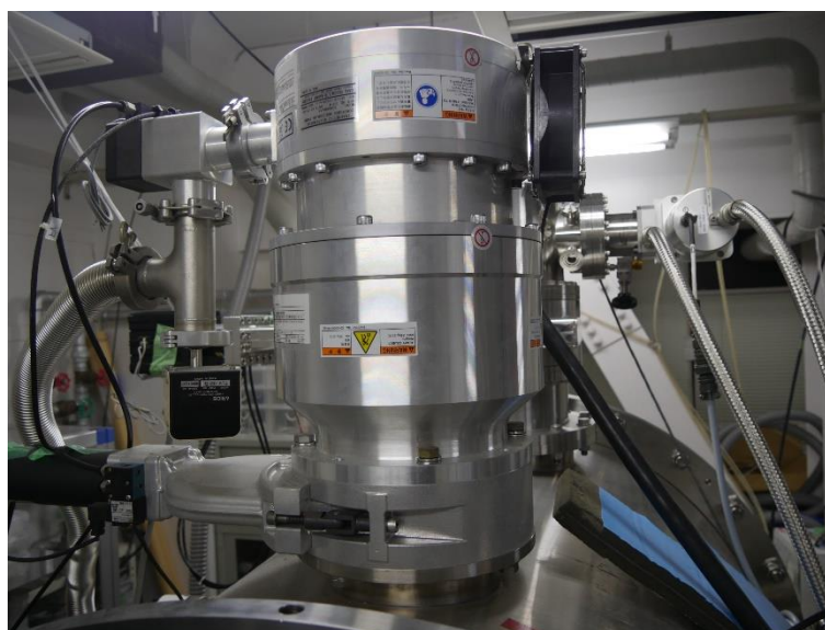
Figure 2-3 Photograph of the turbo molecular pump (OSAKA VACUUM. LTD, model: TG900MVAB) .
