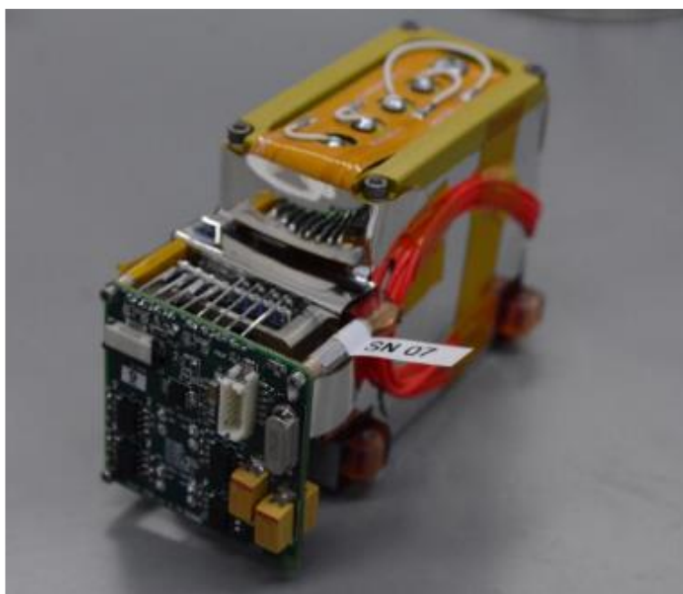
Figure 1-7 Photograph of the steam thruster installed on AeroCube-7B & 7C[118].
