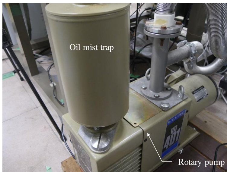
Figure 2-2 Photograph of the rotary pump (ULVAC, model: VD401) .
