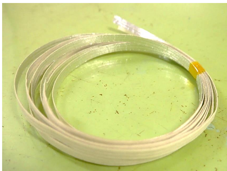
Figure 2-27 Photograph of the tape heater (SAKAGUCHI E.H VOC CORP., model: F-16) .
