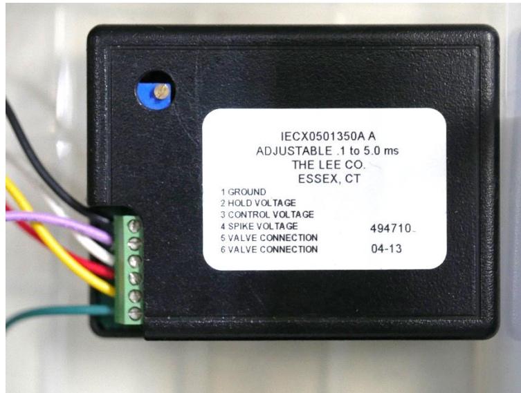
Figure 2-23 Photograph of the valve driver (LEE, model IECX0501350AA) .
