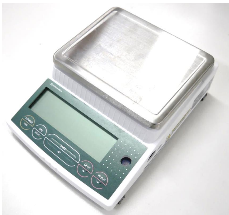
Figure 2-21 Photograph of the mass balance (SIMADU, model: BL-3200H) .
