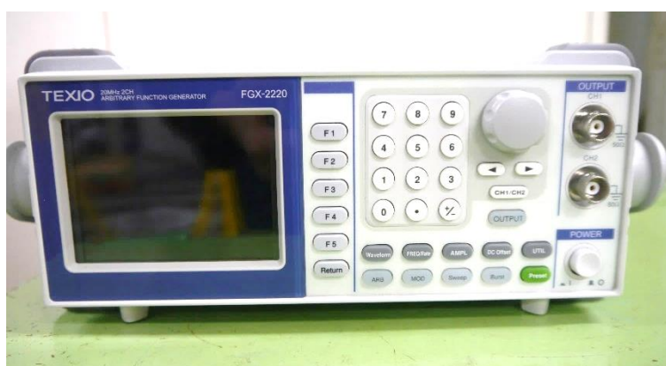
Figure 2-26 Photograph of the function generator (TEXIO, model: FGX-2220) .
