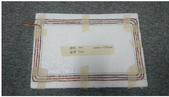
(a) Rectangular coil (Solid wire)
