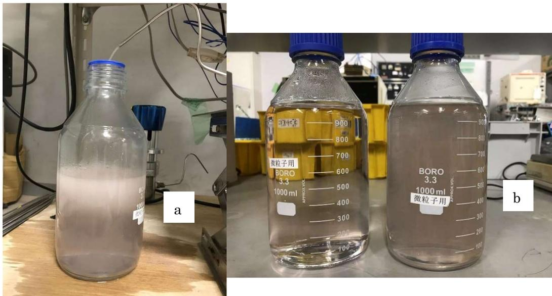
Fig. 3-1. The phenomenon happened in the process of reaction at ethanol ratio 0.1, a) effluent of this reaction, b) comparing between effluent of ethanol ratio at 0 and 0.1.
