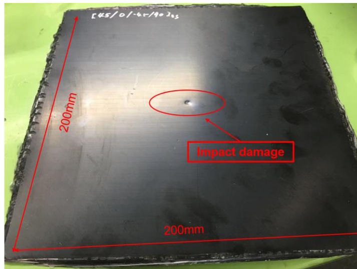
Fig. 2.2. CFRP laminate plate with an impact damage at the center.
