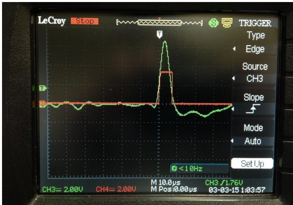
Figure 3.15 Neutron energy signal from a ^{252}\text{Cf} sample measurement with square-shaped signal conversion by comparator.
