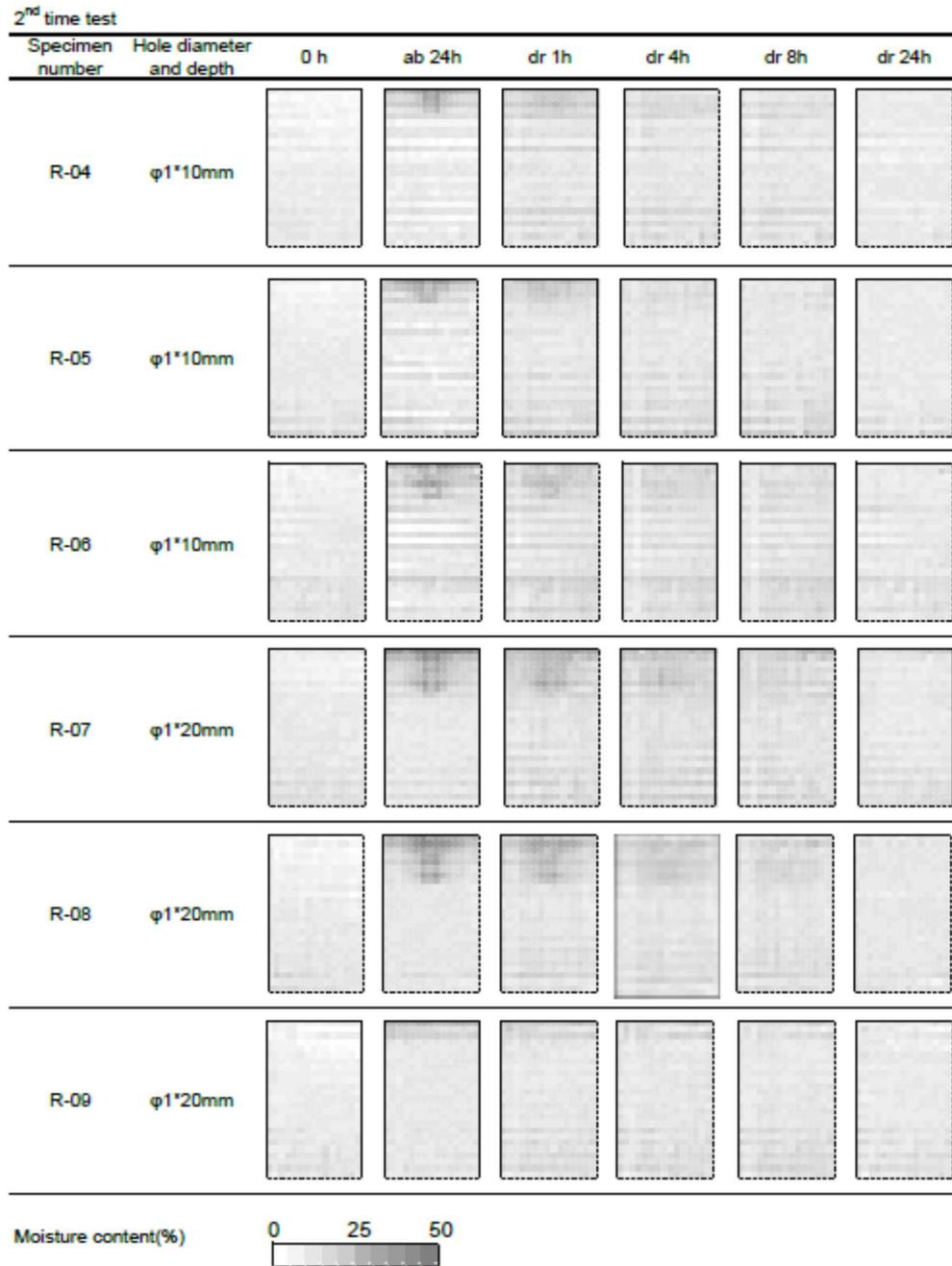
Fig. 6-11 Moisture content distribution of specimens in holes with 1 mm-diameter at the 2<sup>nd</sup> time
