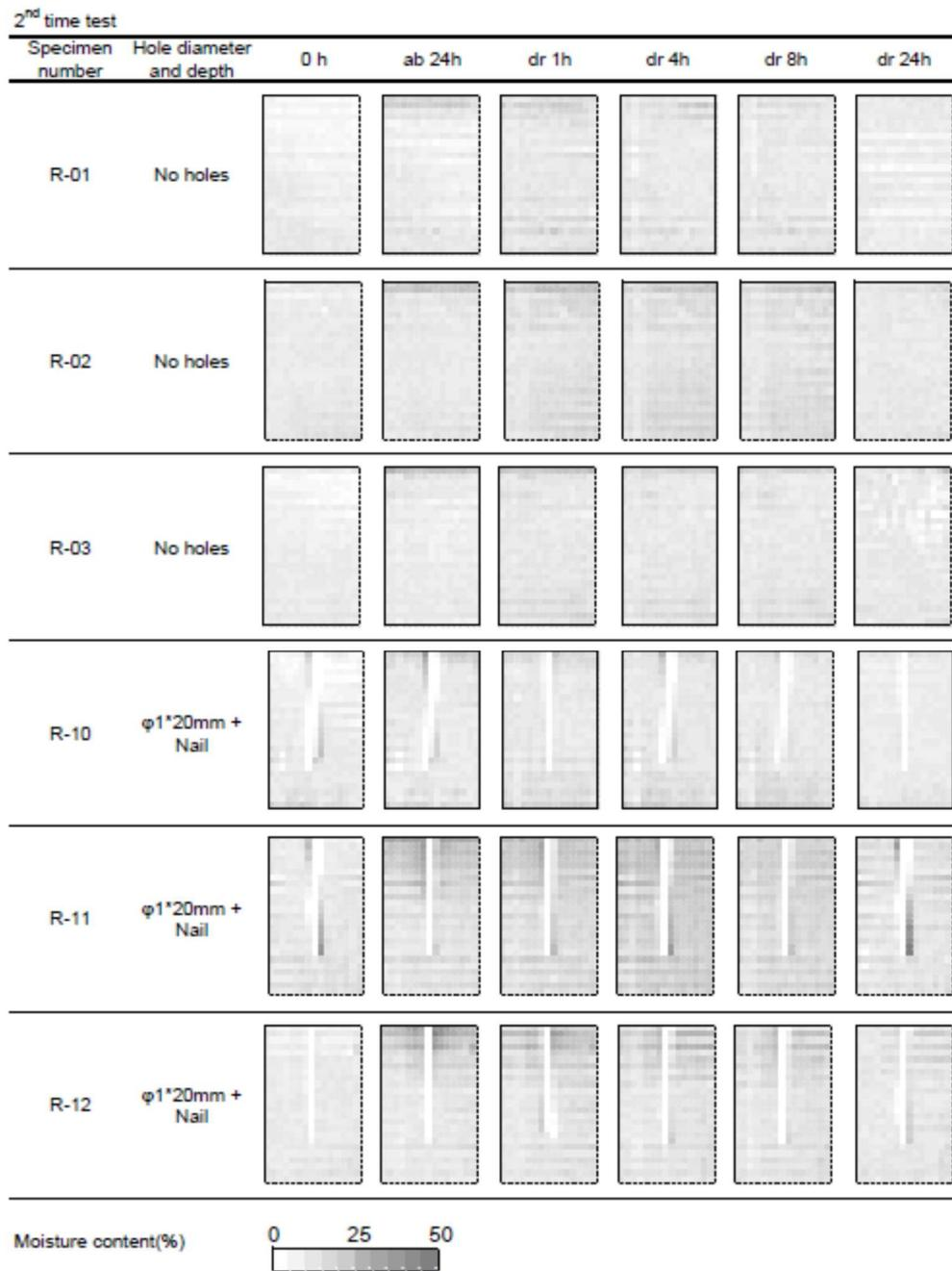
Fig. 6-17 Moisture content distribution of specimens with no holes or with holes and nails at the
