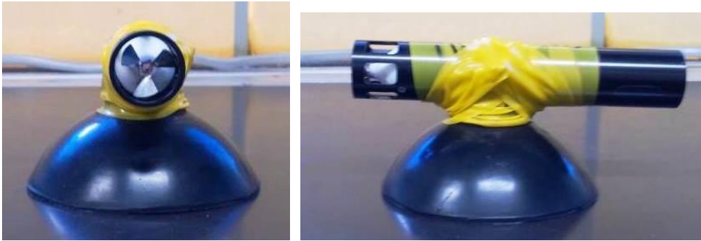
Figure 5-2. W190L-PD3GT accelerometer with black suction cup
