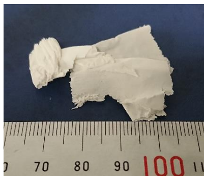
Fig. 3-3 Polymer sorbent mixed with binder
