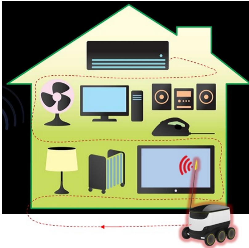
Figure 7.5: A wireless mobile unit going around to collect RSSIs from IoT devices
