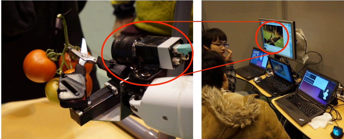
Fig 4.6: Hand camera for the operator to decide whether to cut the tomatoes or whether the hand must get closer to the tomatoes.
