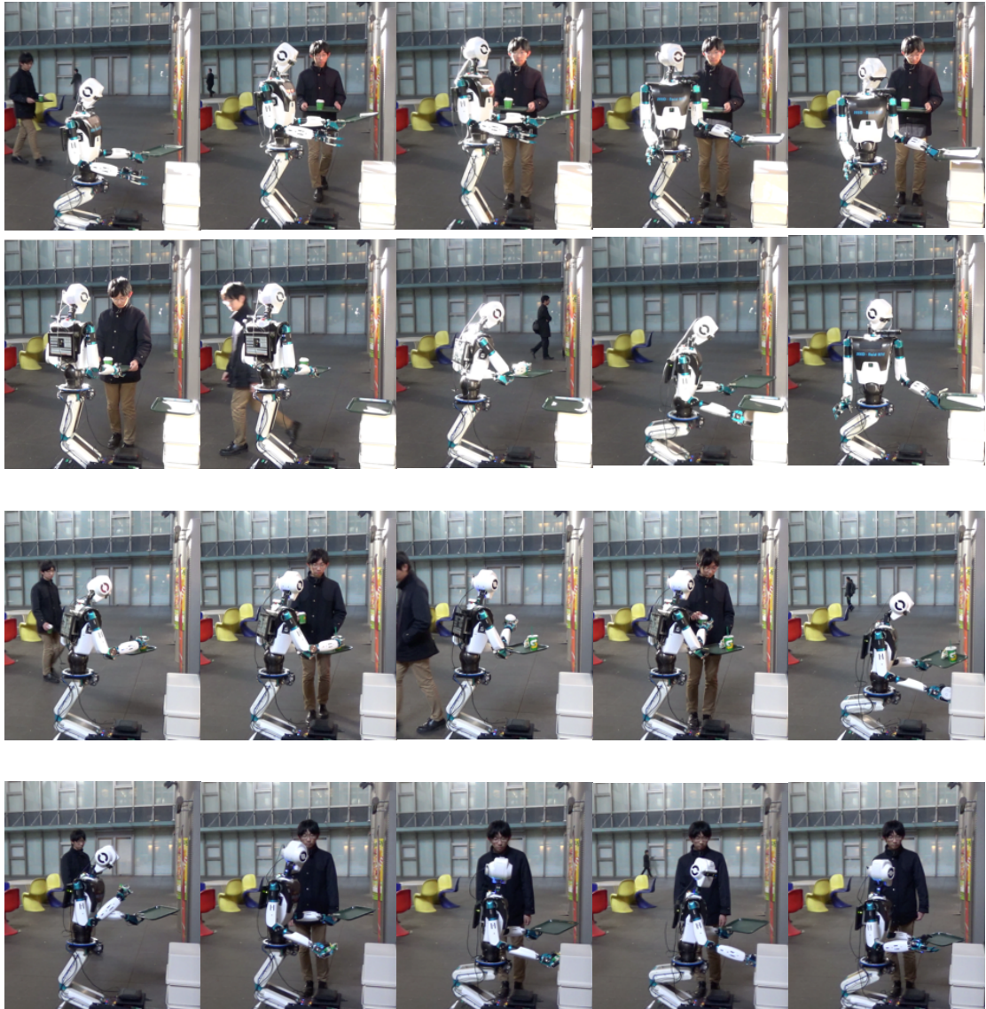
Fig 5.8: An example of a task with different initiation patterns. Top two row shows accepting once and then postponing an interaction to receive a tray. Middle row shows backarding current action to accept an interaction of receiving garbage. Bottom row shows accepting an interaction and then forwarding a task to meet a social context.
