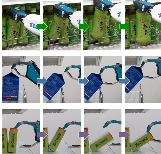
Fig 4.15: Common constraints in picking solved with a combination of the middle mobility layer and grasping modes. [121]
