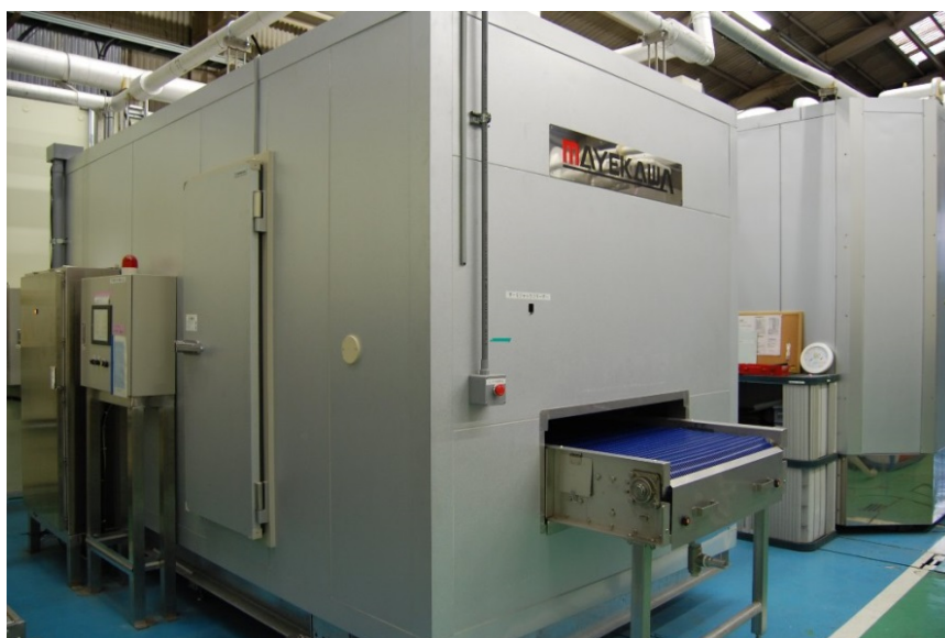
Fig.3-3 Image of impingement freezer
