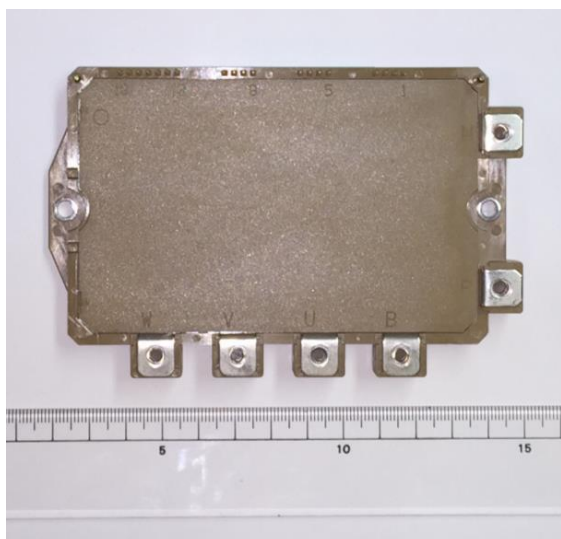
(a) Power device to drive machine tool for automotive power train line (max 160 A(peak))
