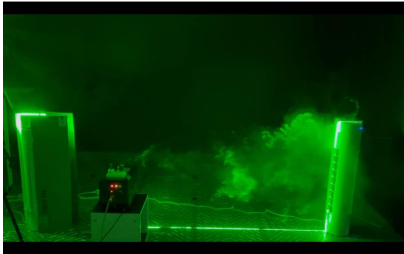
Fig. 4- 24 The smoke diffusion at 4 second when the wind speed of first fan was low-level.
