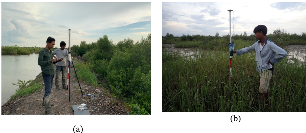
Figure 2.9 Application of PPK in the field;(a) Base station and (b) Rover position
