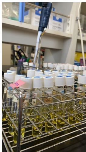
COD test: After 2h heating
