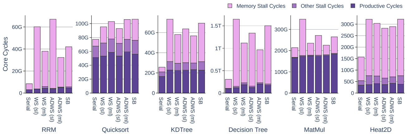
Fig. 5.14.: Breakdown of core cycles profiled by perf system calls.
