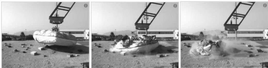
Fig2.14 Landing Test of Vented Airnag[20]
