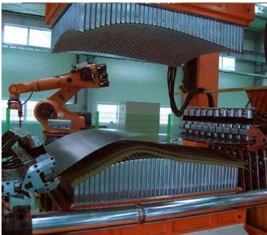
図 43 Multi-Point Stretch-Forming Machine 125
