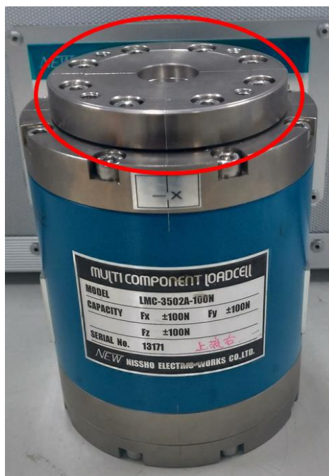
Fig. 4.4 Movable part of load cell [4]
