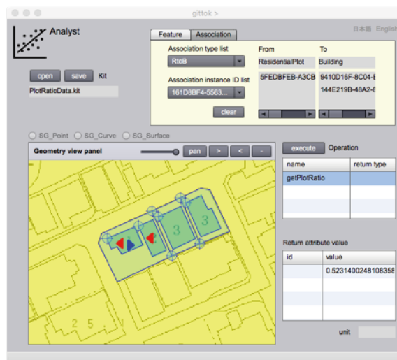
Figure 9.4-2. Execution of operation defined in application schema
