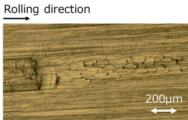
Fig.1-14 Heat scratch occurred on cold rolled strip.
