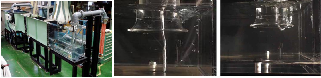
Figure 3.1. Model pump sump (left) and visualized submerged (middle) and air-entrained (right) vortices taken from Okamura et al., 2007 [4].
