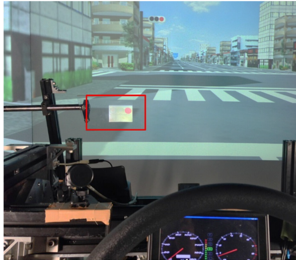
Fig. 4.1. A red signal displayed by the head-up display at a signalized intersection.
