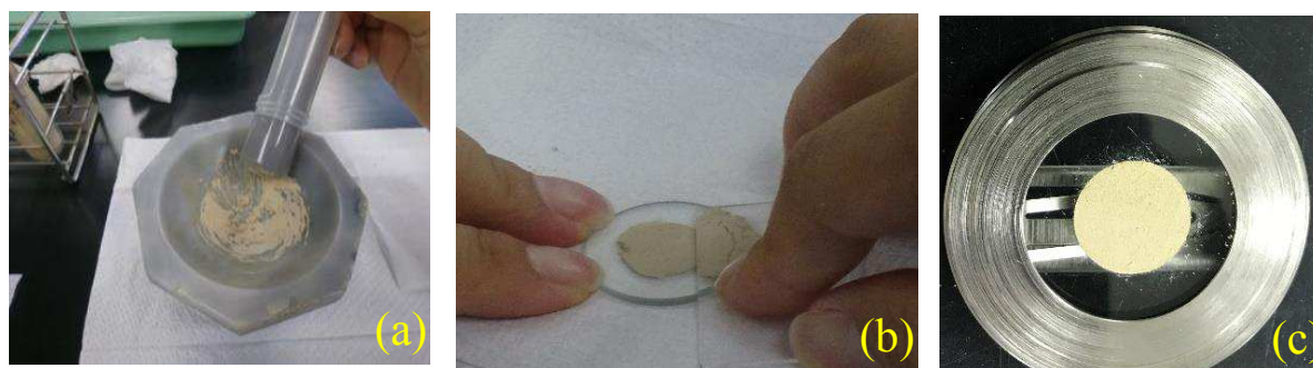
Figure 3:30 (a) Agate mill (b) leveling of the specimen (c) prepared specimen for XRD analysis
