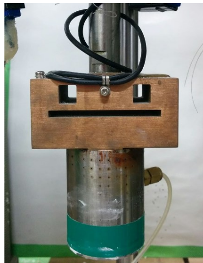
Fig. 2.5. Custom built load cell (triaxial compression machine)
