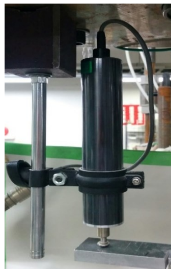
Fig. 2.7. CDP-50 type EDT (triaxial compression machine)
