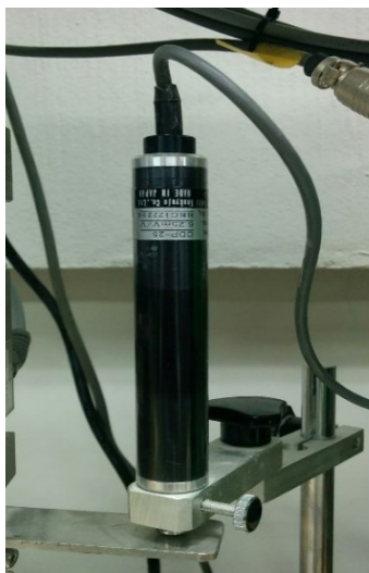
Fig. 2.6. CDP-25 type EDT (unconfined compression machine)
