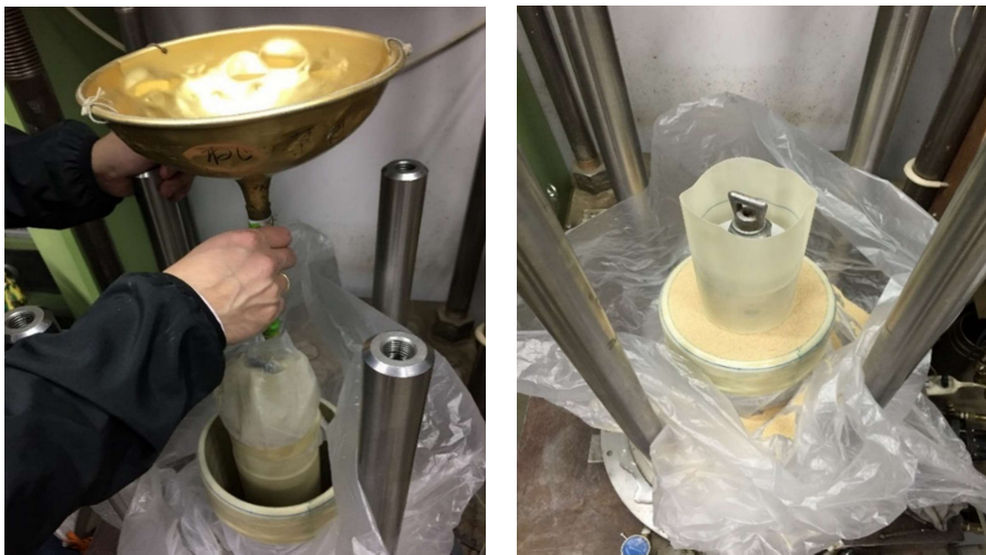
Figure 2.17: Pluviation into the mold
