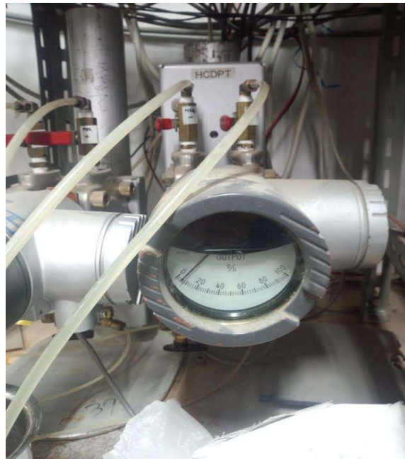
Figure 2.9: High Capacity Differential Transducer (HCDPT)
