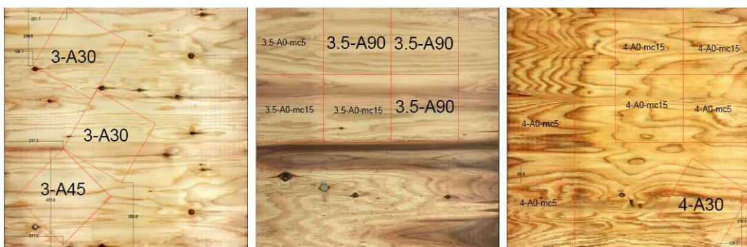
Figure 3-4. Examples showing typical drawings on layer of each thickness. Each sample was labeled with thickness followed by fiber orientation.
