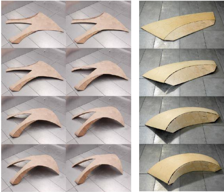
Figure 2-5. Left: combination of 12mm beech wood with glass fiber textile of 80g/m 2 . Thickness of each elemental pieces were robotic milled to achieve the curvature. Right: combination of 10mm maple and 2.0mm spruce.
