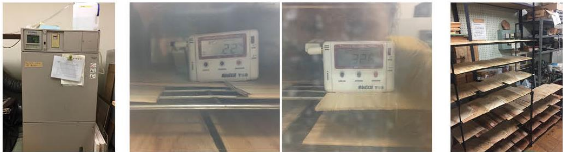
Figure 3-5. Left: climate chamber for equilibrate active layers. Center: condition of oven to dry the restrictive layers to 5%. Right: condition to dry restrictive layers to 12%
