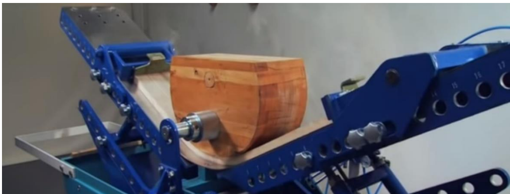
Figure 1-5. Automated steam bending. Bending requires much external energy, equipment and force. (GHEBavaria, 2012)
