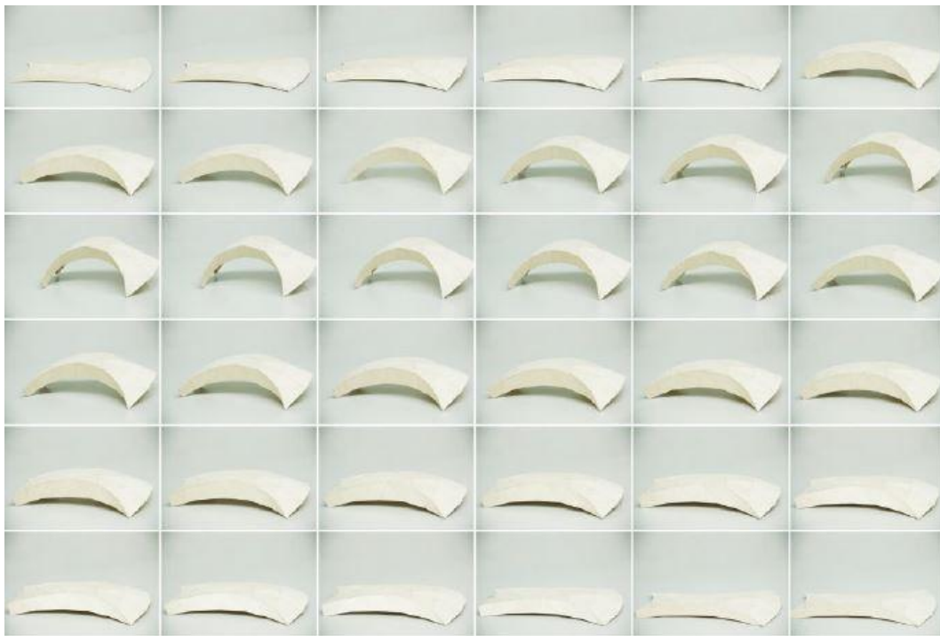
Figure 2-4. Research by Wood and Menges. Small scale experiment using 1.2mm maple veneer and glass fiber textile of 40g/m 2 . The relative humidity was oscillated for 1-hour cycle between 30% and 60%. (Wood, Correa, Krieg & Menges, 2016).
