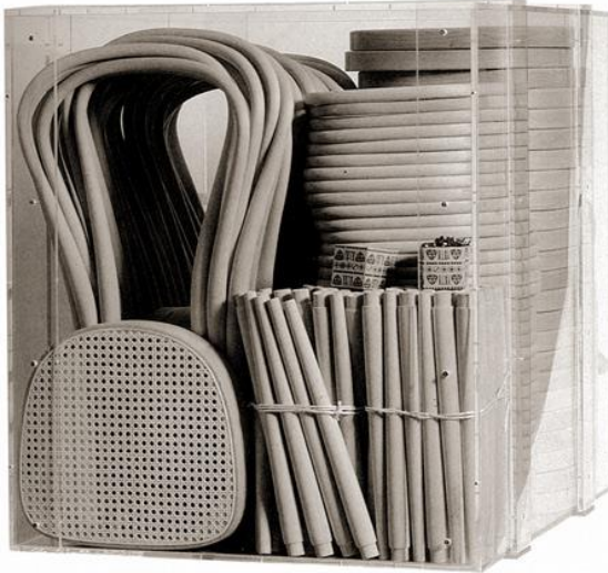
Figure c. Thonet Chair mass produced in 1850s, denoting the standardization of wood bending technology. (THONET, n.d.)
