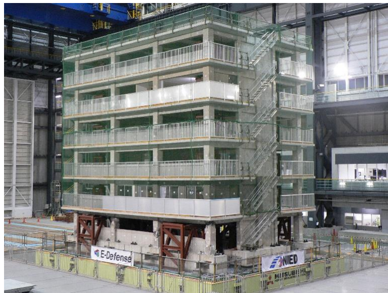
Figure 3-18 Six-story RC shear wall building test model
