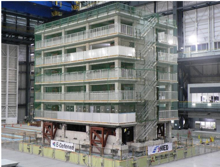
Figure 4-6 Tested building model
