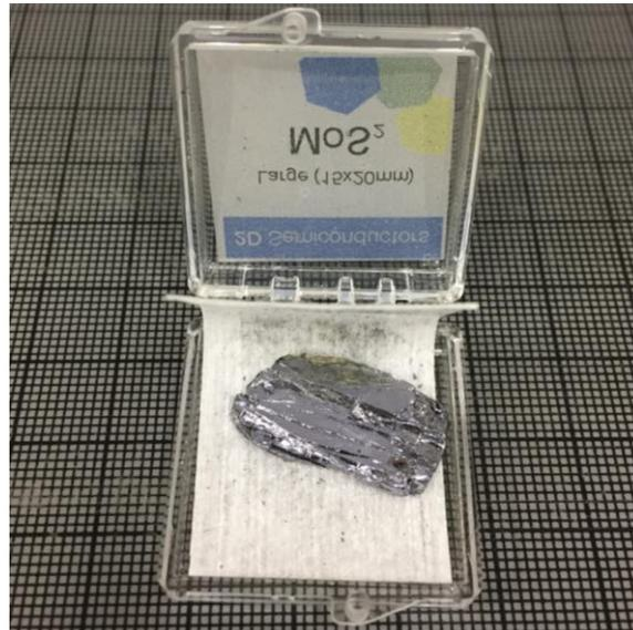
**Figure 1.7 Photograph of a piece of bulk MoS<sub>2</sub> crystal, which was purchased from 2D Semiconductors Inc.**
