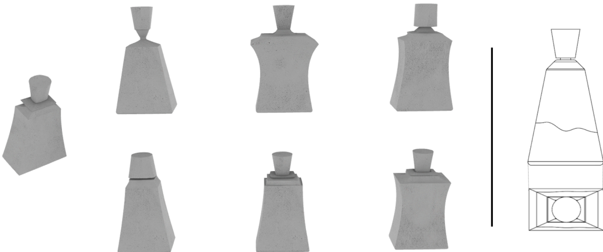
Figure 4.31: Bottle samples created with sweep method using 2 profile curves and multiple closed cross-sections.
