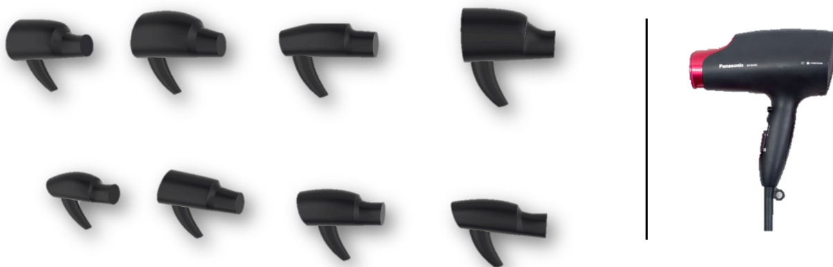
Figure 4.29: Hairdryer samples generated by sweeping a single closed cross-section.
