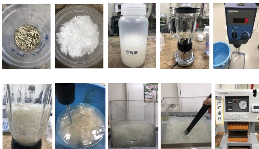
Figure 3-13 Manufacturing process of the AP and CF/AF paper
