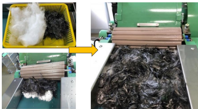
Figure 2-2 The opening and mixing of CF and PA fibers
