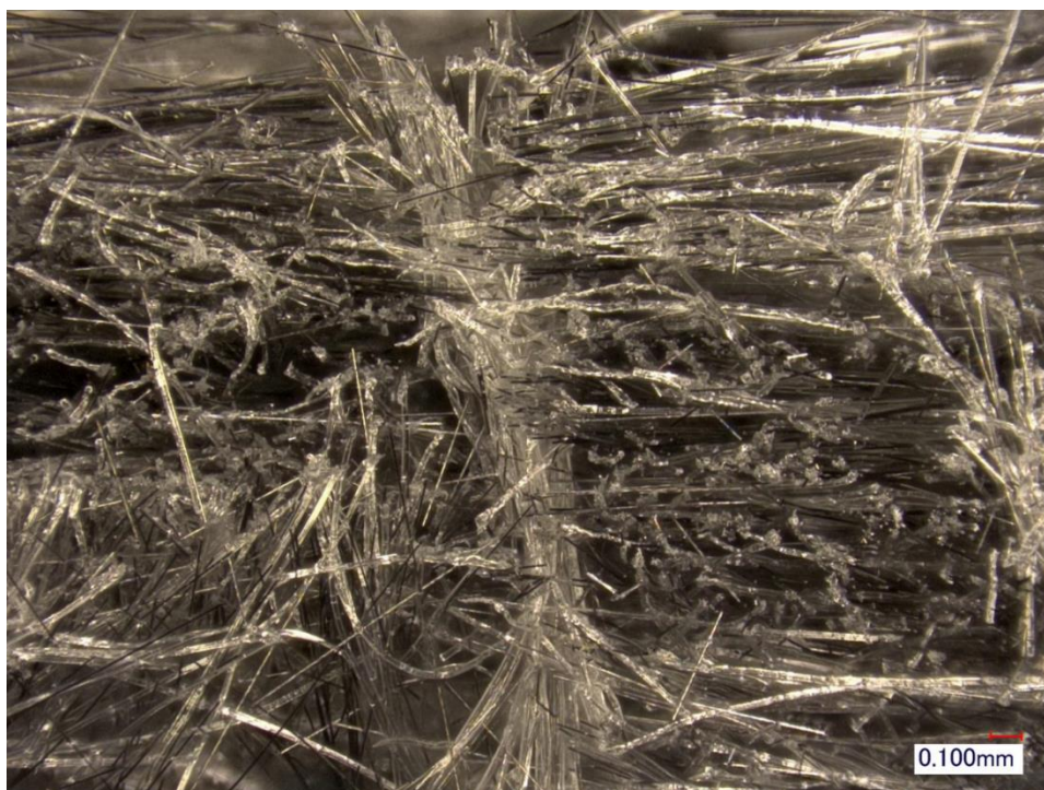
Figure 4-13 Optical microscopy image of the cross-section of a needle-punched CPT sheet
