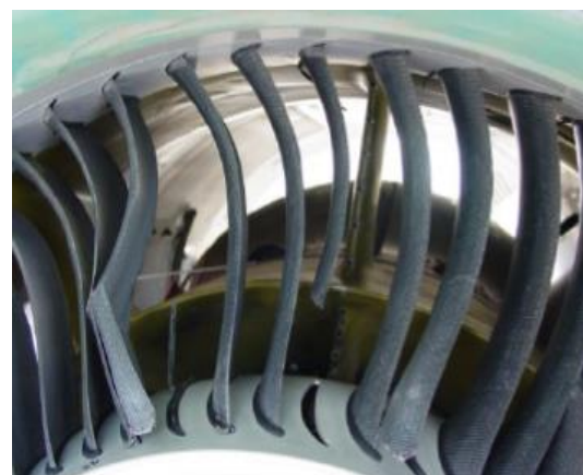
Figure 1.2 Catastrophic damage in stator [2]
