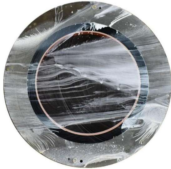
Figure B.11 Tip clearance flow (oil flow)
