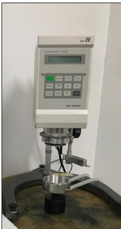
Fig. 3.8. Viscometer used for the rheological analysis
