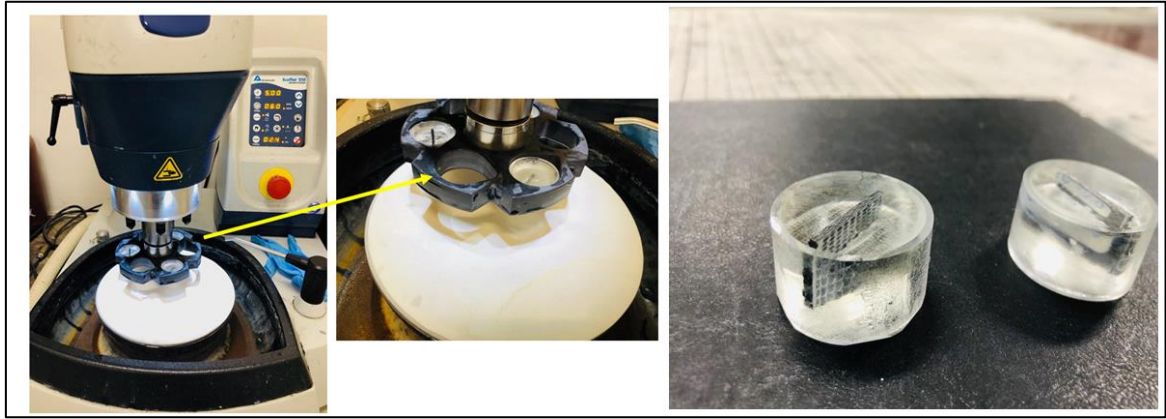
Fig. 6.8. The polisher used for the sample preparation and the samples prepared using clear rings and clear epoxy.
