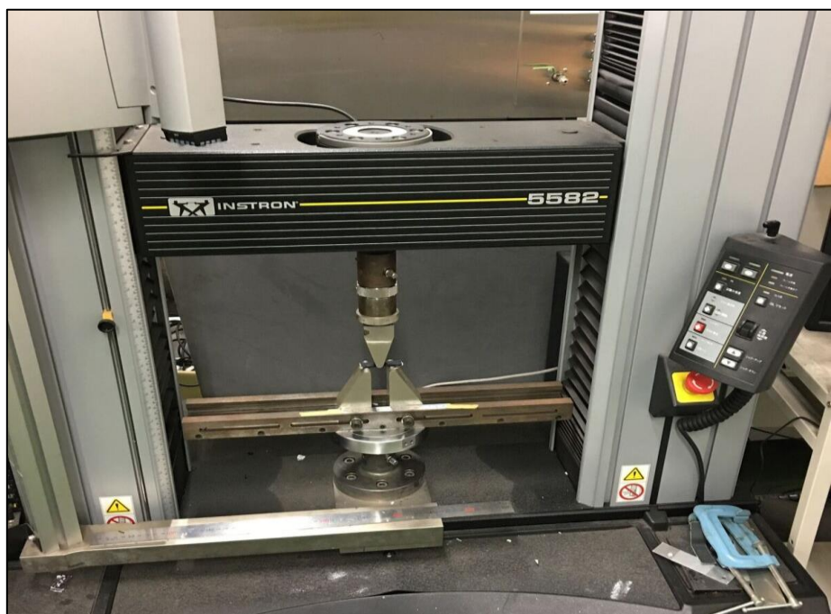
Fig. 3.10: The UTM for conducting flexural tests on the composites.
