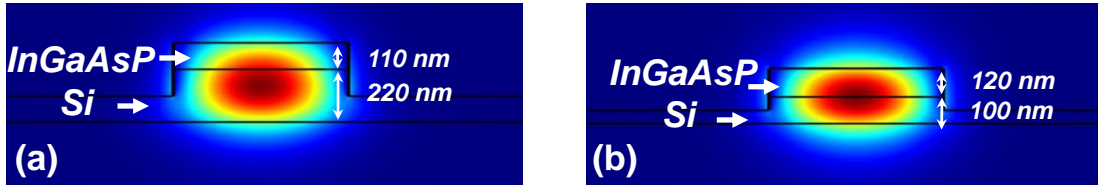
Fig. 3.11. The TE fundamental mode of III-V/Si hybrid MOS optical phase shifter with varying thickness of InGaAsP and Si layer.
