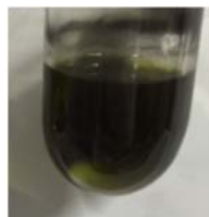
Figure 3-34. Pd black precipitation when the reaction to synthesize 2a from 1a proceeded for three hours using Pd(TFA) 2 .
