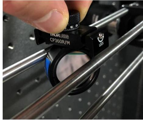
(b) Removing optical elements
