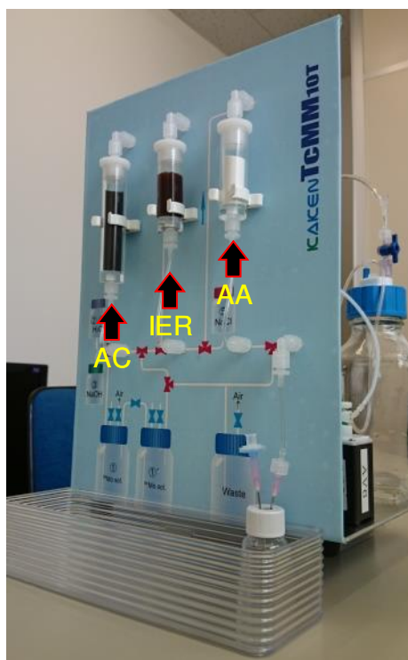
Fig. 7.3. (a) ^{99}\text{Mo}/^{99\text{m}}\text{Tc} adsorption characteristics of alumina and activated carbon. (b) A prototype AC chromatographic device. AC: activated carbon; IER: ion exchange resin; and AA: activated alumina. Figure (b) courtesy of Kaken Inc., Japan.
